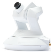
Indoor Wireless P/T with 350° Rotation (ADC-V620PT)
